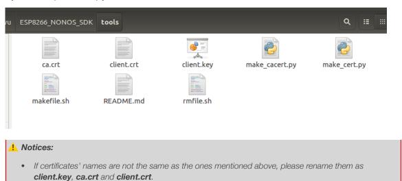
Then run the *makefile.sh* to generate certificates for the SSL encryption.
